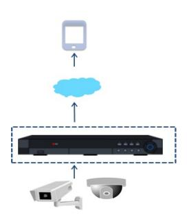
With a traditional system, the video processing and management occurs on a computer installed at your site.
