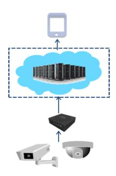
With a true cloud solution, the video processing and management is performed by the cloud. The system may have an onsite device to communicate. with the cameras and the cloud, but the device is simple and acts as a communications conduit.
